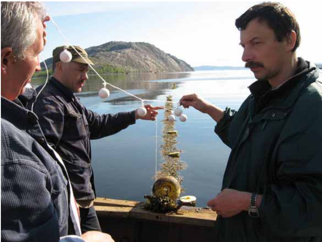
Fig. 10 Preparation for monitoring of hydrodynamic regime using plaster balls
